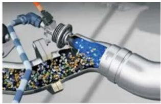
Fig. 5.a. The organisation of the post-treatment system of exhaust fumes for Audi Q7
