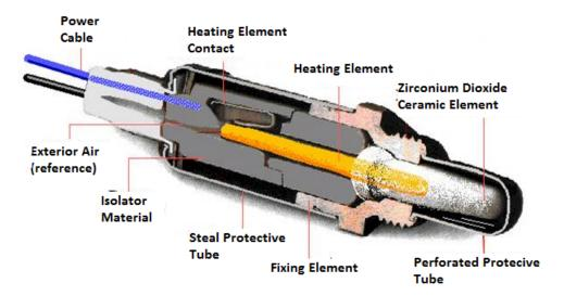
Fig. 4. Self-heating lambda sensor
