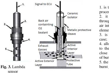
1. is the connection cable to the process computer;
