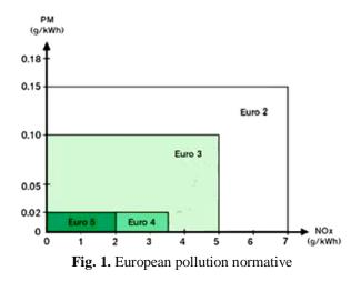
The hereto figure presents a diagram which indicates the measure in which the European norms reduce the  $NO_x$  and particles emission.
